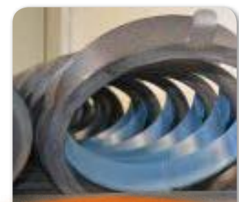
Freehanded rubber coating on nearly every surface
